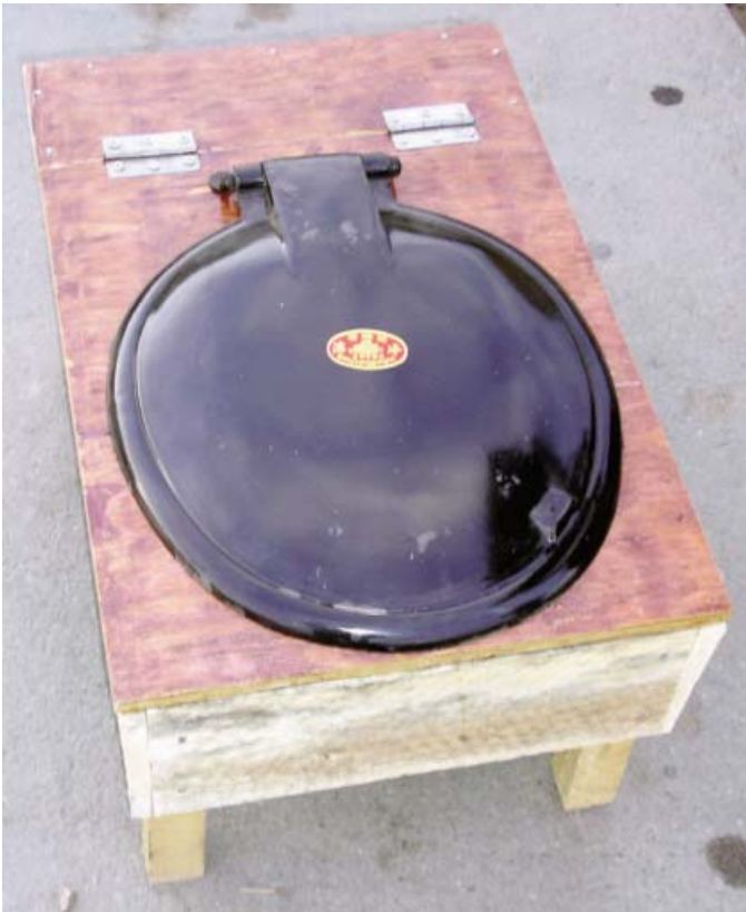
The bio-toilet itself is a simple, inexpensive collection device.
