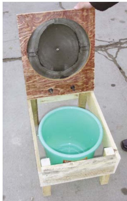
The bio-toilet itself is a simple, inexpensive collection device.
