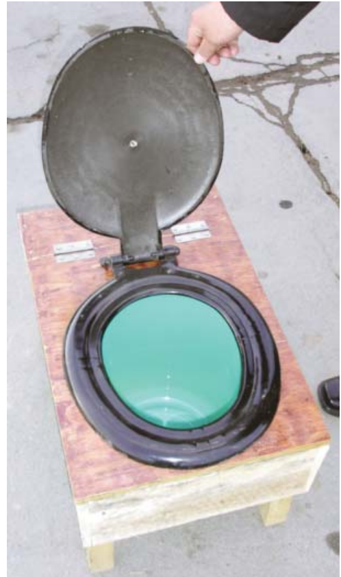
The bio-toilet itself is a simple, inexpensive collection device.
